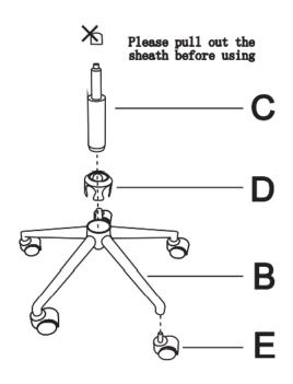
STEP 3: Put the Part from step 1 on the Part from step 2
